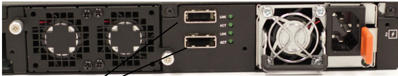
Figure 3-13. N3048 Mini-SAS Stacking Ports Close-up
